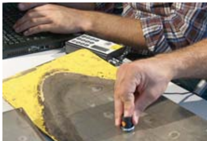
Researchers measured the thickness of the Deere forager's DuraLine coatings with an Echometer probe, to test DuraLine's effect.
