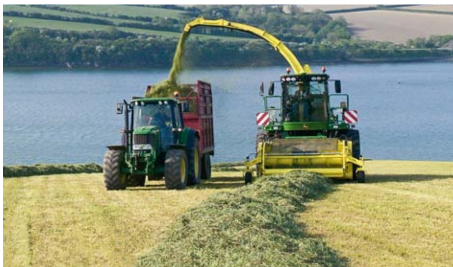
The small but high-yielding grass fields of Cornwall, England, saw the Deere 7750i forager performing at its most economical. Fuel consumption dropped to as low as 0.37 litres/t of fresh mass.
