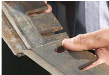
Maize knives were changed after chomping through 96,000t of crop. One grass knife was swapped after completing 32,000t.
